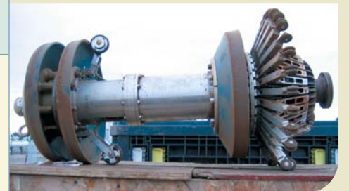
This portly 'smart pig' was placed inside a water makeup pipeline between Suncor's Oil Sands and Firebag locations earlier this year. His job is to detect dents, wrinkles, or other anomalies in the line. This pig and others on his team work to strengthen the integrity of the pipelines by tracking data that can be used to minimize the risk of ruptures.
