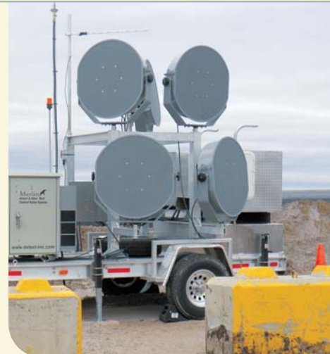
The LRAD unit is a compact, focused planar speaker array that can project out to half a mile with verbal commands and digital recordings.
