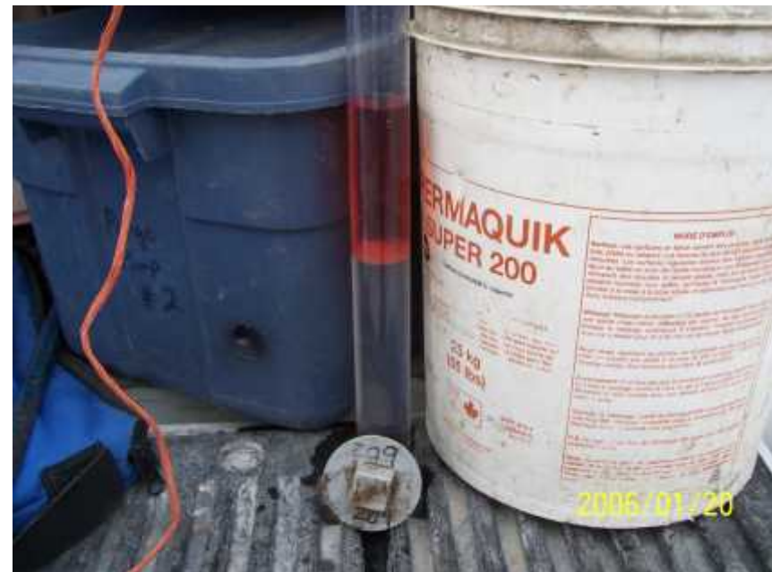
LPH in monitoring well bailer.
